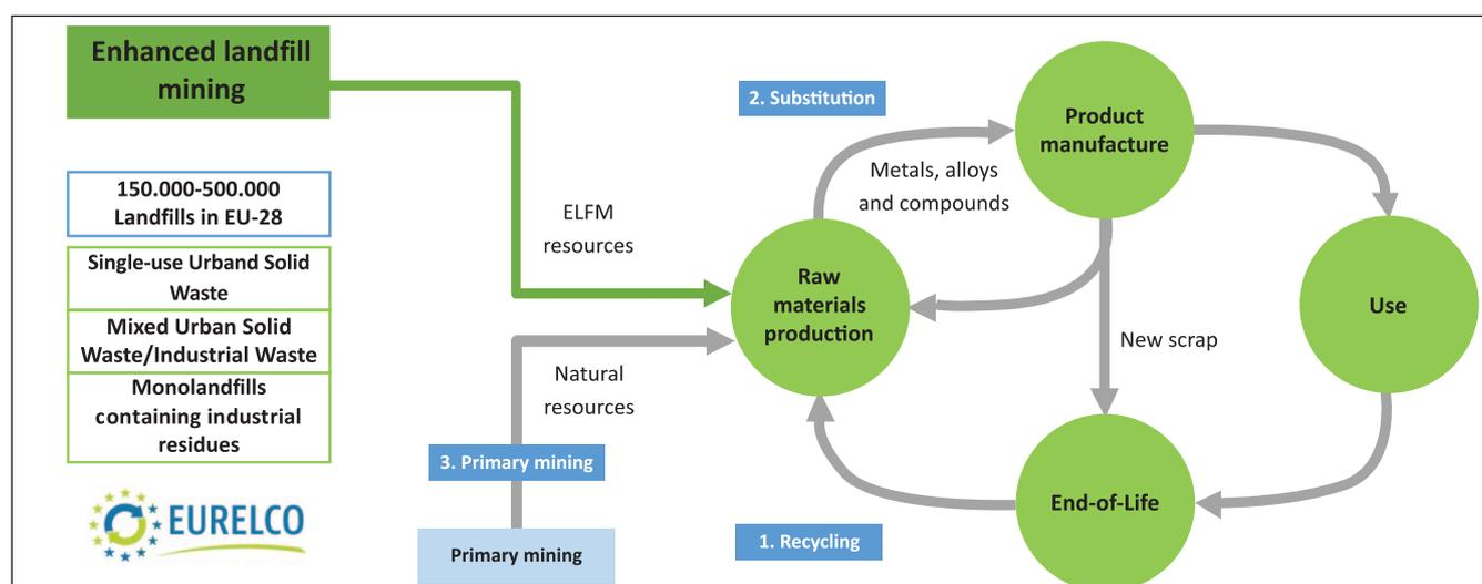
Comprehensive raw materials programme. ELFM adds additional 'postponed' circularity by re-integrating previously landfilled resources into the materials cycle. Figure adapted from C Meskers (Umicore)
